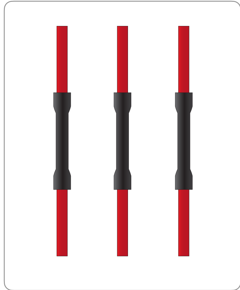
Non-Sealing Butt Connectors (allows for moisture and corrosion)
