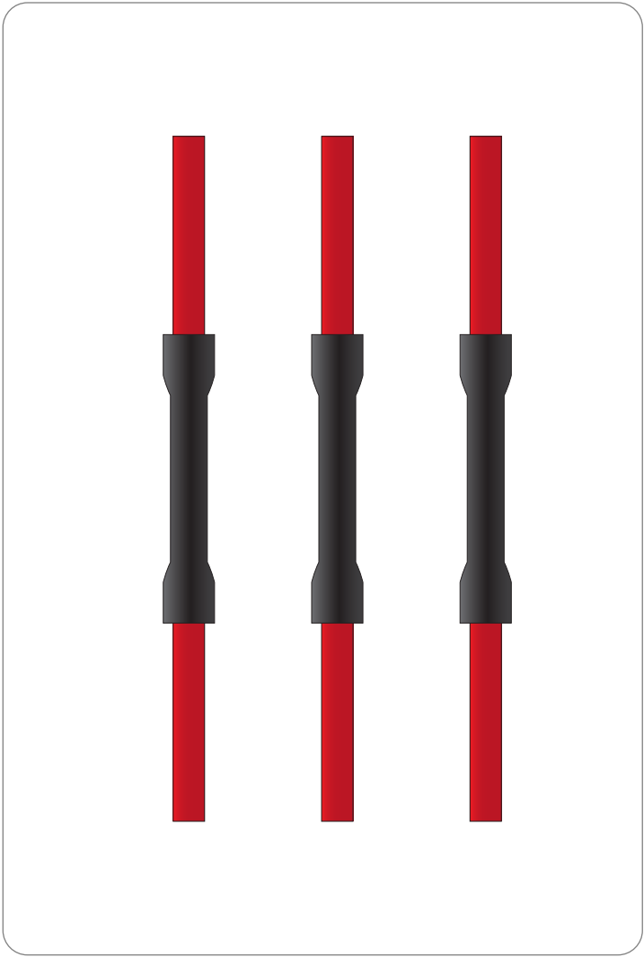
Non-sealing butt connectors (allows for moisture and corrosion)
