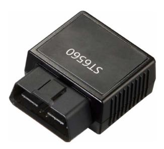
The ST6560 is a full-featured 4G vehicle tracking solution that plugs directly into a vehicle's OBD II port to track GPS location and capture engine diagnostics data, including DTC codes, RPMs, vehicle speed, and more. A three-axis accelerometer also supports harsh event detection, including harsh acceleration, braking, and cornering.
